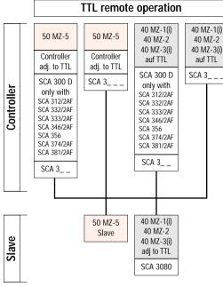
Here, "remote operation" means cordless firing of additional (slave) flash-
